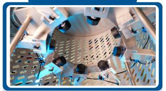
The multidiameter head adapts to a wide range of tube sizes without adjustment. Perfect for agile, multi-SKU production lines.
