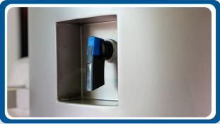
Designed with hygiene and safety in mind, the recessed control panel protects key functions from moisture, debris, and accidental activation — ensuring reliable operation and easy cleaning in demanding food production environments.
