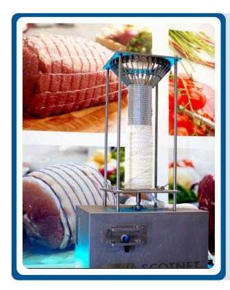
The **Scotnet Auto Net Loader** is a highspeed netting system designed to optimise throughput, reduce manual handling, and improve overall packaging efficiency.
